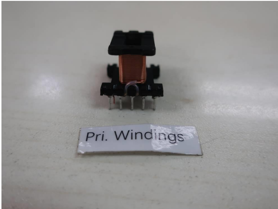
Internal view-7 of transformer T1
