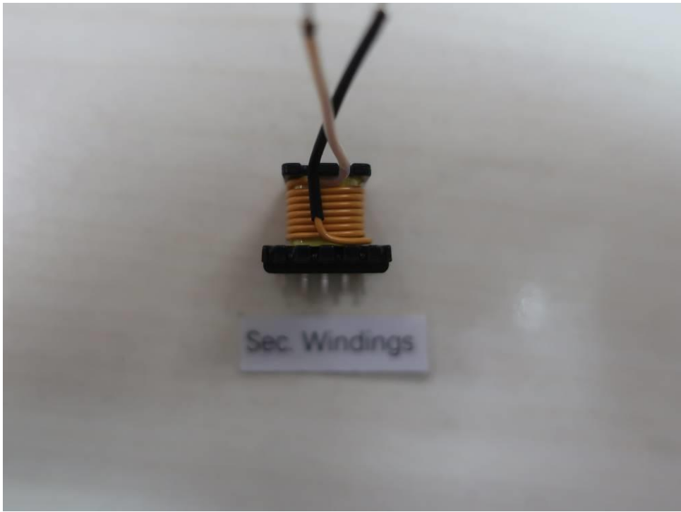
Internal view-4 of transformer T1
